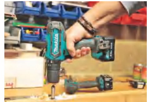
Checking the power, the driver was able to drill 25mm holes with a Forstner...
